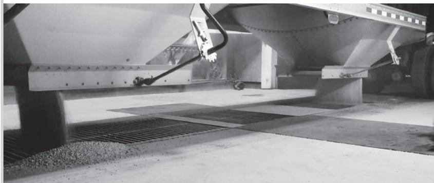
The all new Dual Hopper Chain Conveyor takes system capacity to the next level, by allowing both trailer hoppers to unload at the same time. The Dual Hopper Chain Conveyor features an impressive 10,000 BPH capacity and matches the capacity of the 12" Double Run, 12" Grain Pump Loop, Low Profile Chain Conveyor and Mass-Ter Mover Chain Conveyor. The Dual Hopper Chain Conveyor dramatically reduces unload times and increases harvest efficiency.
